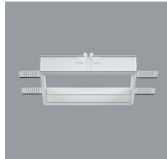
82923.000 Mounting frame For flush mounting of luminaires with ceiling aperture 206x206mm. Polymer, white (RAL9002). Mounting for ceiling thicknesses of 12.5-25mm. The recess depth of the luminaire increases by 2mm. Weight 0.30kg
