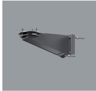
34955.000 Cantilever arm for standing luminaire installation on upright supporting pole ø 60-89mm or wall. Housing: stainless steel. Graphit m, powder-coated. Clamping plate or second cantilever arm for fixing on upright supporting pole to be ordered separately. Upright supporting pole ø 60-89mm to be ordered separately. Weight 2.20kg
