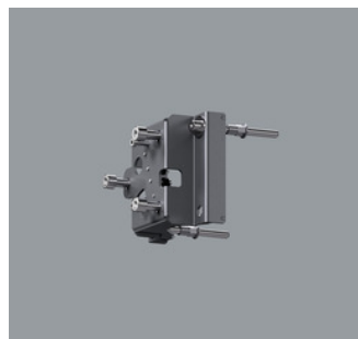
34953.000 Attachment for upright supporting pole ø 60-89mm. Housing: stainless steel. Graphit m, powder-coated. Clamping plate or second attachment for fixing to be ordered separately. Upright supporting pole ø 60-89mm to be ordered separately. Weight 1.00kg
