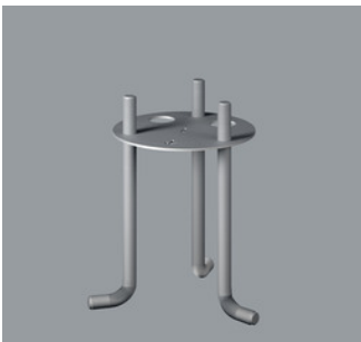
33981.000 Concrete anchor Mounting plate with threaded bar and fixing nuts M10. Individual parts to be assembled on-site. Weight 0.76kg
