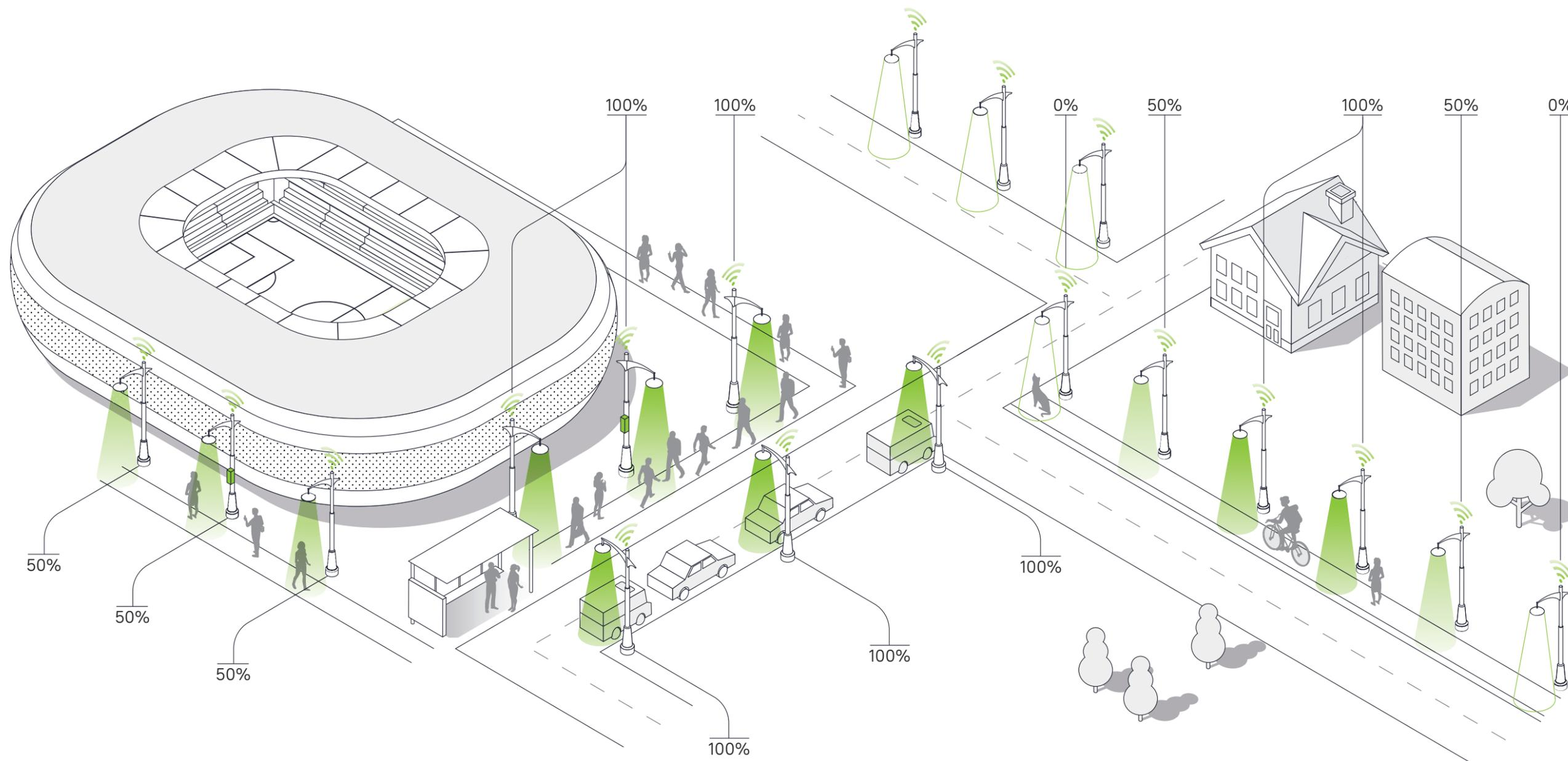
The volume-based light control solution from esave makes your lighting system even more intelligent. The lighting system is equipped with sensors to detect traffic density. When it recognizes increased traffic density (e. g., during the rush hours or for a special occasion such as football match) a higher level of light intensity will automatically be activated, providing better visibility and safety.
