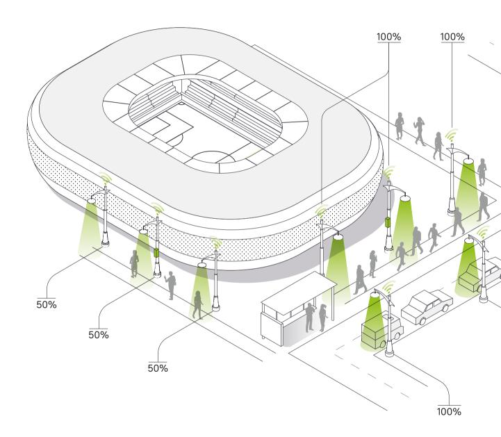
The volume-based light control solution from esave makes your lighting system even more intelligent. The lighting system is equipped with sensors to detect traffic density. When it recognizes increased traffic density (e. g., during the rush hours or for a special occasion such as football match) a higher level of light intensity will automatically be activated, providing better visibility and safety.
