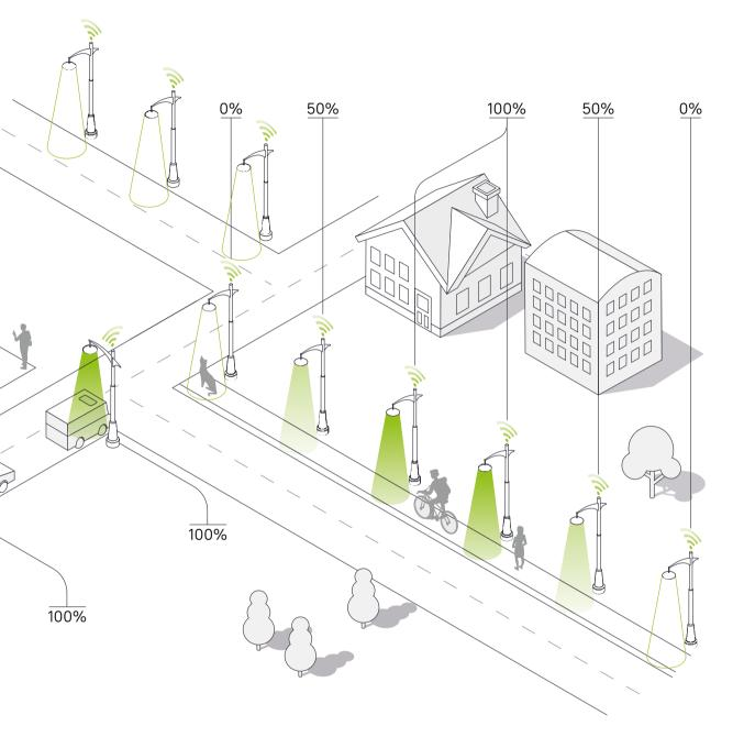
The idea behind esave's Light on Demand solution is very simple: Each luminaire is equipped with a motion sensor that registers whether there is traffic on the street or not. Once the sensor registers analogue movement in the illumination area, light intensity is automatically increased to a higher level and a message is sent to the next luminaire(s), which also increase light intensity before the pedestrian or vehicle reaches the next luminaire position.
